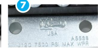
Precision manufacturing techniques ensure critical tolerances are met. Divider valves and baseplates are laser etched with the Ariel logo.
