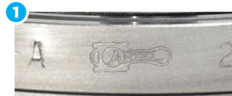
Built specifically for the reliability and efficiency of high-speed compressors, genuine Ariel valves are etched with the Ariel logo, and the part numbers are roll-stamped along the outer edge of each seat and guard.
