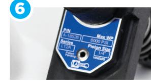
Ariel's redesigned force-feed lubricator pumps improve priming and lower camshaft rolling resistance. Identify your genuine Ariel pump, size and part number on the blue data tag.
